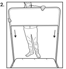
Locate the Sign by inserting the Stand tube into the sign tube
