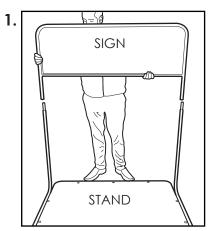
Position the Sign above the Stand and align the tubes
