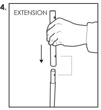
For extended stand, insert the Extension tube between the Stand and Sign
