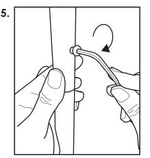
Secure the Sign to the Stand (and Extension) using the M6 Screws
